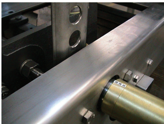
Figure 1.2 - Safety Solenoid and Slotted Plate
