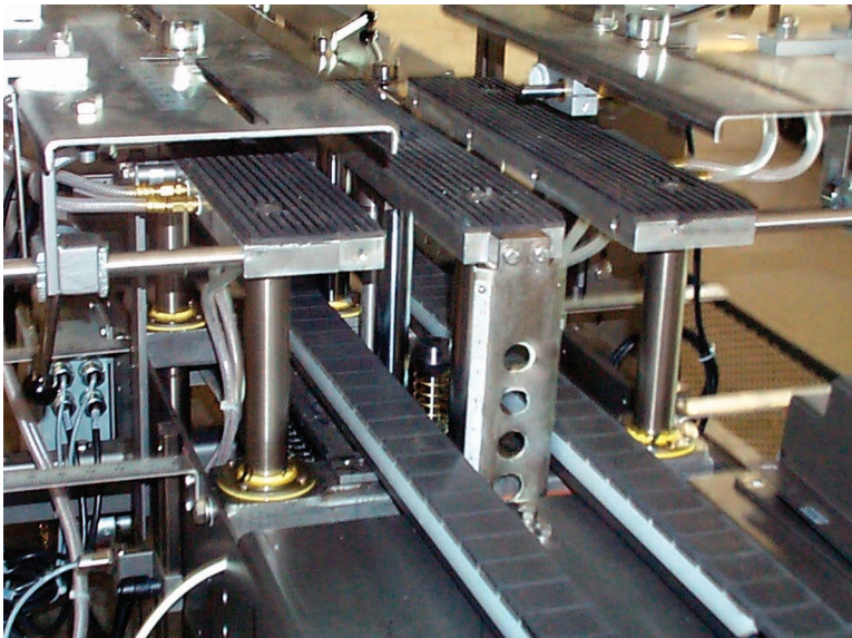
Figure 1.1 - Case Packer Lift Table (Shown in the up and locked position)
