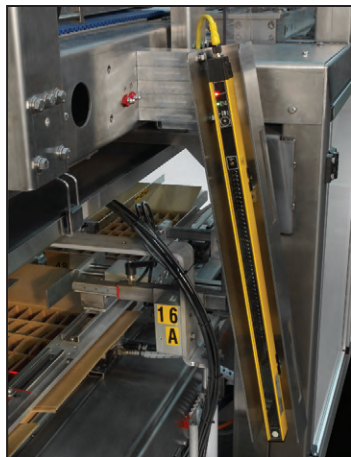
Light curtains enable quick access and protection
